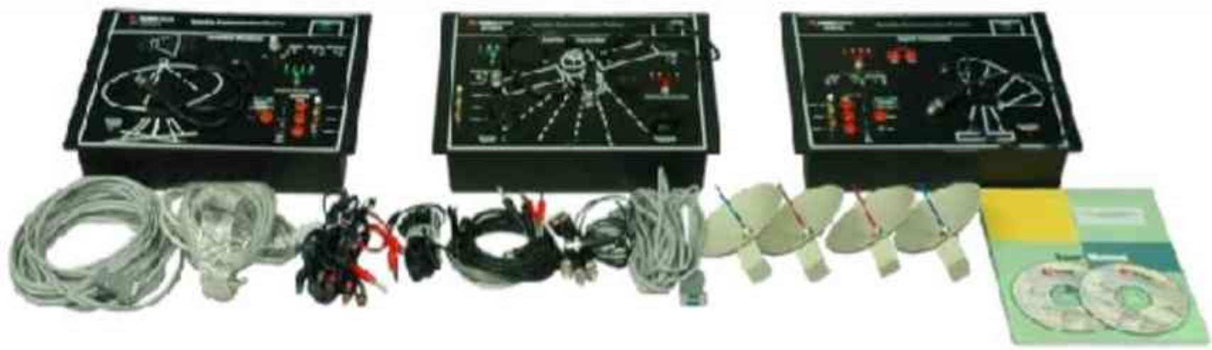
Uplink, Downlink and Satellite Transponder.
